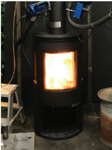
The stove on the test rig, output test
